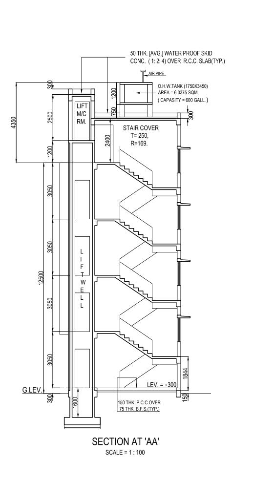
NOTES & SPECIFICATIONS: ALL DIMANSIONS ARE IN MM. UNLESS OTHERWISE MENTIONED. THE DEPTH OF SEPTIC TANK AND SEMI U.G. WATER RESERVIOR SHALL NOT EXCEED THE DEPTH OF NEAREST BUILDING FOUNDATION. GRADE OF CONCRETE = M20, AND GRADE OF STEEL = Fe 500.
